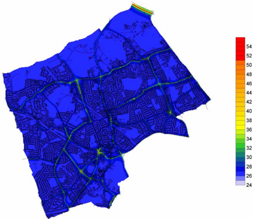
Map 2. London Borough of Harrow - Number of days with daily mean PM10 exceeding 50 microgrammes per cubic metre ( \mu\text{g}/\text{m}^3 ) for 2004 based on 1996 meteorology (from 10)
