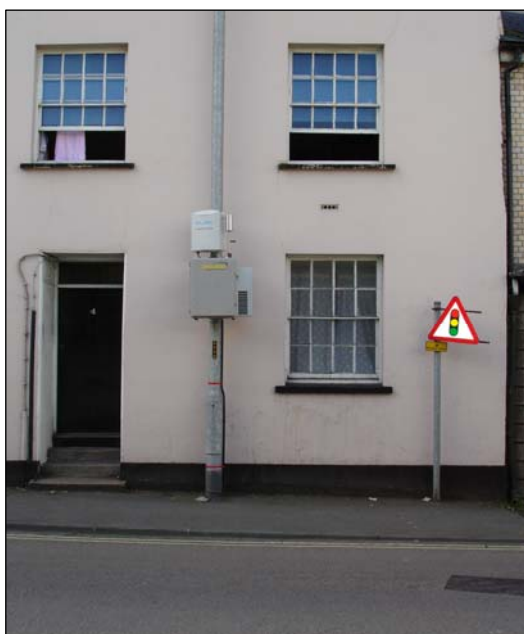
Plate 2. AirPointer continuous NO 2 monitor located in Dennison Rd.
